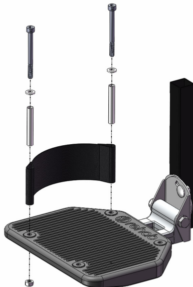
Diagram 1. Assemble the screws, washers, tubes, heel loops, foot plate and nuts according to the figure. Use an Allen key (5 mm). Tighten the screws securely.
